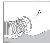
Advice: If the hose is long and the room temperature low, the moisture might condense to water inside the hose. This is an unavoidable natural phenomenon. To prevent this water from lying in the hose or flowing back into the tumble dryer, it is advisable to drill a small hole (dia. 3 mm) in the lowest point of the hose and to place a small container below it.(See picture, point A).
